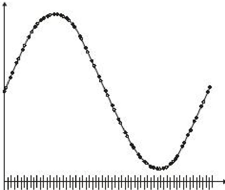
$$V_{\text{rms}} = \sqrt{\frac{\sum_{i=1}^N V_i^2}{N}}$$
