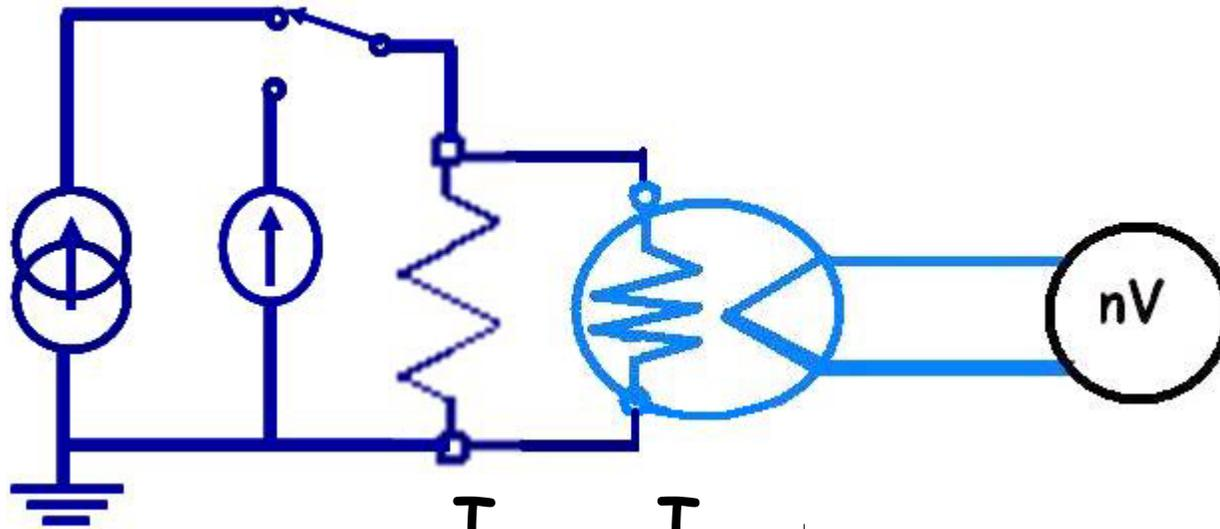
$$\delta = \frac{I_{c.a.} - I_{c.c.}}{I_{c.c.}} \Big|_{E_{c.a.} = E_{c.c.}}$$
